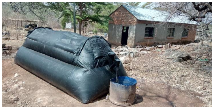
Above: A biodigester, filled with gas on the top layer, ready for use at Thulani Farms.
