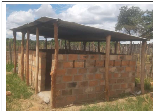
Calf pen building – shade, ventilation and protection from wind and rain
